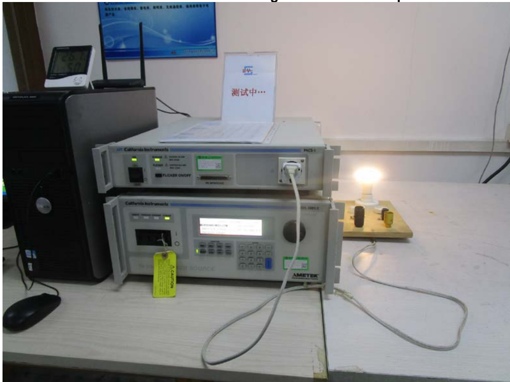
Current Harmonics /Voltage Flicker Test Setup
