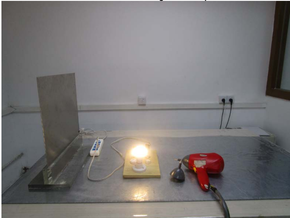
Electrostatic Discharge Test Setup
