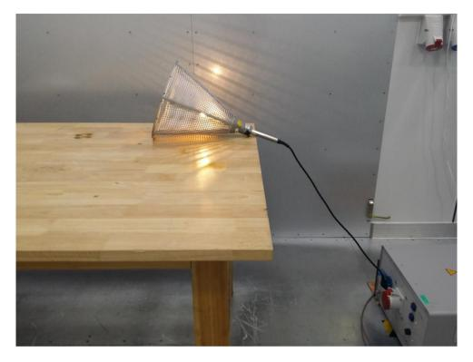
Test Setup: Radiated Emissions (Magnetic Field: 9 kHz-30 MHz)
